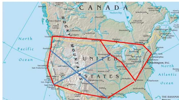
**Figure 4: Hybrid North American HVDC Supergrid**
